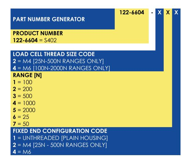
Example: A 1000N Load Cell with an M6 Thread and M6 Housing
