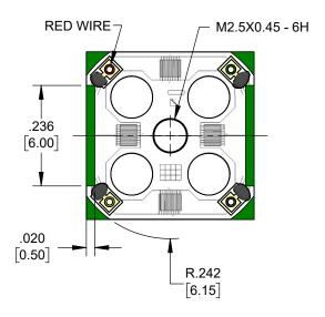
NOTE: THE S410 DOES NOT HAVE ANY MOUNTING HOLES. TO IMPROVE LINEARITY, THE SENSOR CAN BE WELDED TO A FLAT AND RIGID "MECHANICAL GROUND" PLANE ALONG ITS BOTTOM EDGE, OR CLAMPED DOWN IN THE AREAS SHOWN IN GREEN ABOVE.
