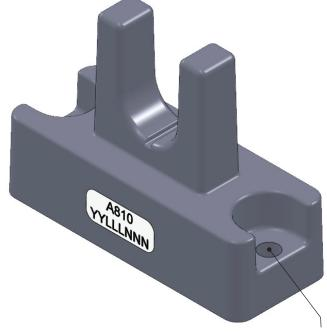
Mounting features designed for #4-40 for M2.5 Threaded inserts in bosses on mating panel
