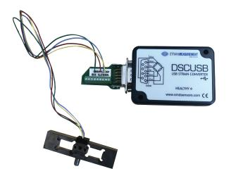
The E370 **DSCUSB** is a compact, high performance strain gauge digital signal conditioner with USB connectivity aimed at applications which require high-accuracy measurement and repeatability.
