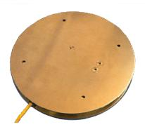
Designed for a semiconductor corrosive gas delivery tool, The **W200 Scale** was required to fit into a tight envelope (under 6" in diameter and less than 1" tall). Constructed of 300 series stainless steel, this scale also needed to offer I<sup>2</sup>C communication output data and be accurate to 0.1% of full scale or just 5 grams. With a temperature rating up to 70C, the effect on accuracy due to temperature was required to be less than 0.02% of full scale, or 1 gram.
