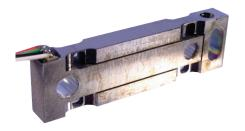
The **S256 Load Cell** uses proprietary sputtered thin film strain gauge technology to create a rugged sensor with exceptional long term stability. These sensitive gram range load cells are manufactured using state-of-the-art equipment. The compact sensor with it's integral overload protection scheme can be used to electronically measure force or displacement in a wide variety of applications.
