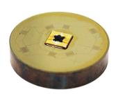
The Series **940 Pressure Sensor** is a stainless-steel wetted surface pressure diaphragm with a proprietary sputtered thin-film full-bridge strain gauge circuit. The sputtered metal strain gauge circuit offers superior long term stability and higher temperature capability than other strain gauge technologies. A unique lead out pad design provides ease of soldering and rugged construction. The 10K ohm bridge offers low power consumption for transmitters. Ideal for pressure transducer OEMs.
