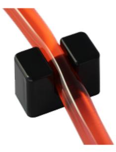
The A830 Air-In-Line/Bubble Detector is one of our standard sensors for use with most 1/2 inch OD tubing. It uses our proprietary digital noninvasive ultrasonic bubble sensing technology to accurately and reliably detect bubbles in a wide variety of fluids in rigid or soft tubing materials. Custom characteristics can be provided for OEM users.
