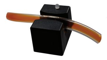
The A430 Bubble Detector is one of our standard sensors for use with most 1/4 inch OD tubing. It uses our proprietary digital noninvasive ultrasonic bubble sensing technology to accurately and reliably detect bubbles in a wide variety of fluids in rigid or soft tubing materials. Custom characteristics can be provided for OEM users.
