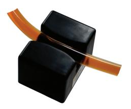
The A330 Air-In-Line/Bubble Detector is one of our standard sensors for use with most 3/16 inch OD tubing. It uses our proprietary digital noninvasive ultrasonic bubble sensing technology to accurately and reliably detect bubbles in a wide variety of fluids and tubing materials. Custom characteristics can be provided for OEM users.
