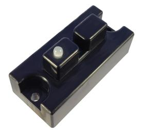
The **A240 Bubble Sensor** is one of our standard sensors for use with most 1/8 inch OD tubing. It uses our proprietary digital noninvasive ultrasonic bubble sensing technology to accurately and reliably detect bubbles in a wide variety of fluids in rigid or soft tubing materials. The A240 uses a smaller area along the tube for easy and repeatable tube insertion. Custom characteristics can be provided for OEM users.
