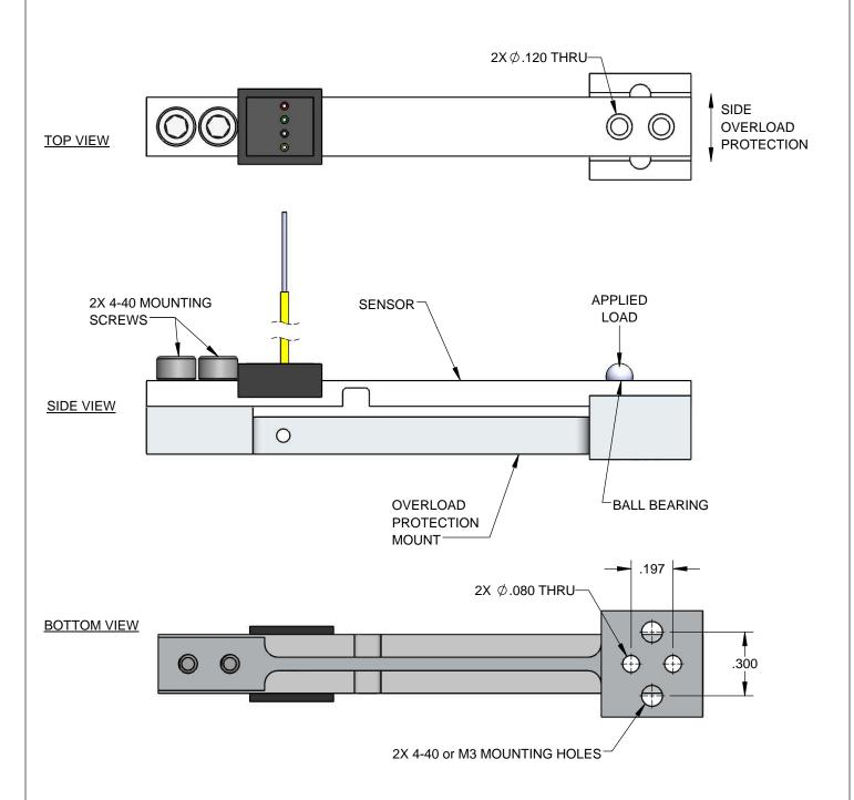
The overload protection mount is mounted to mechanical ground.
