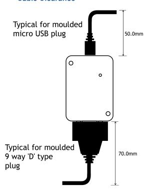
These are typical clearances but smaller moldings or using a tighter cable radius can reduce this.
