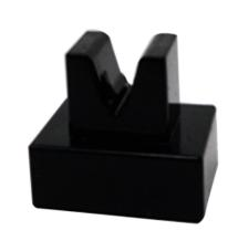
Strain Measurement Devices Solution: To address this problem, Strain Measurement Devices has designed a custom bubble sensor. This bubble sensor is based in SMD's proprietary ultrasonic detection technology. The sensor utilizes a "v-shaped" tube slot to allow for east and automated tube installation. Each sensor is custom calibrated with customer selected tubing to selectively detect unsafe bubbles and ignore nuisance bubbles, based on customer specifications.
