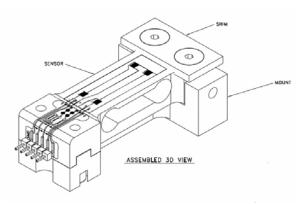
SMD manufactures a family of low force range (450 grams to 9Kg) center point load cells that are made for small size platform scales typically no larger than 9 X 9 inches. Obviously the lower range force sensors are more likely to get overloaded so we also make a unique mounting that will make these sensors almost unbreakable. These mounts will allow the sensor to see up to 10X Full Scale load in compression and tension. They also provide a great deal of side load and torsion protection.
